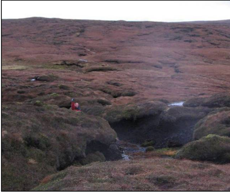
Figure 31 Example of a peat gully, Turbine C41 (HU 4300 6478). At this point, the measured peat depth was 0.2m and the gully depth was 2m, giving a processed peat depth of 2.2m.
